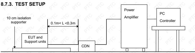
For the actual test configuration, please refer to the related item – Photographs of the Test Configuration Note: 1) The EUT is setup 0.1 m above Ground Reference Plane
